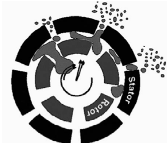
Figure 1.12: Rotor-stator shear by spinning shaft, inside view [25].
